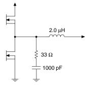
Figure 18. Filter Components
