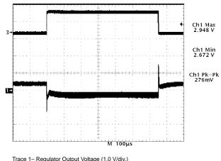
Trace 1– Regulator Output Voltage (1.0 V/div.) Trace 2– Regulator Output Voltage (20 V/div.)
