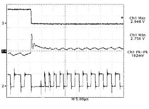
Trace 1– Regulator Output Voltage (1.0 V/div.) Trace 2– Inductor Switching Node (5.0 V/div.) Trace 3– Output Current (13 to 0,5 Amps) (20 mV/div.)
