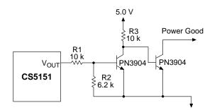
Figure 15. Implementing Power Good with the CS5151
