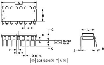
NOTES: 1. DIMENSIONING AND TOLERANCING PER ANSI Y14.5M, 1982. 2. CONTROLLING DIMENSION: INCH. 3. DIMENSION L TO CENTER OF LEADS WHEN FORMED PARALLEL.
