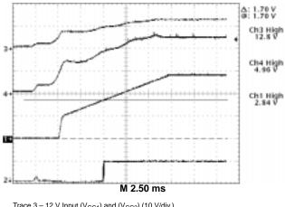
Trace 3 – 12 V Input (V<sub>CC1</sub>) and (V<sub>CC2</sub>) (10 V/div.) Trace 4– 5.0 V Input (2.0 V/div.) Trace 1– Regulator Output Voltage (1.0 V/div.) Trace 2– Power Good Signal (2.0 V/div.)
