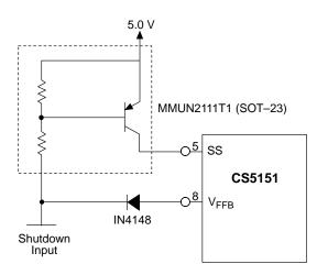
Figure 14. Implementing Shutdown with the CS5151
