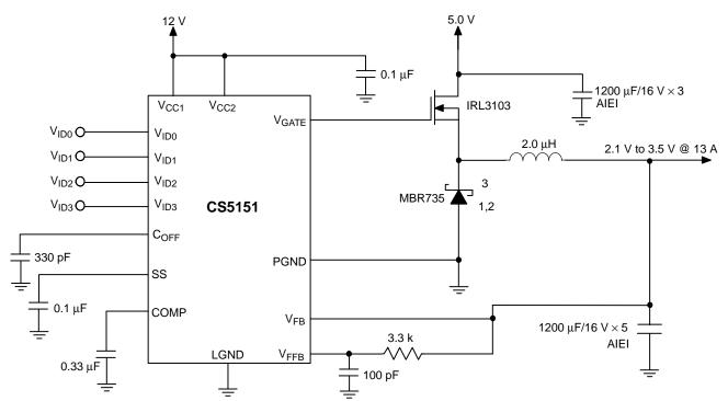
Figure 1. Application Diagram, Switching Power Supply for Core Logic – Pentium<sup>®</sup> Pro Processor with MMX Technology
